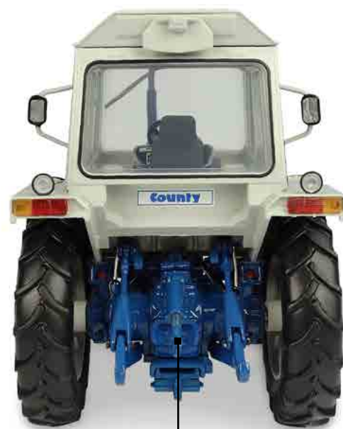
Third point linkage adjustable New standard realistic UH coupling system
