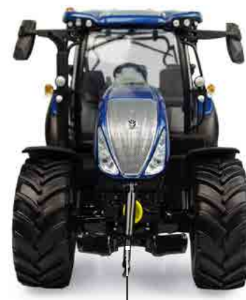
Adjustable 3 points linkage
