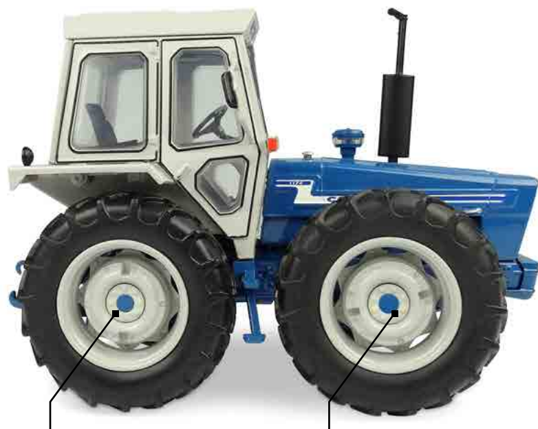
Wheel weights are fitted as standard on County 1174 to obtain maximum tractive.
