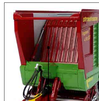
Sloping perforated front wall
