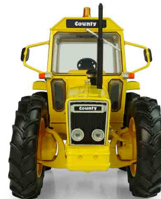
Specific front hood with headlight in the front grille
