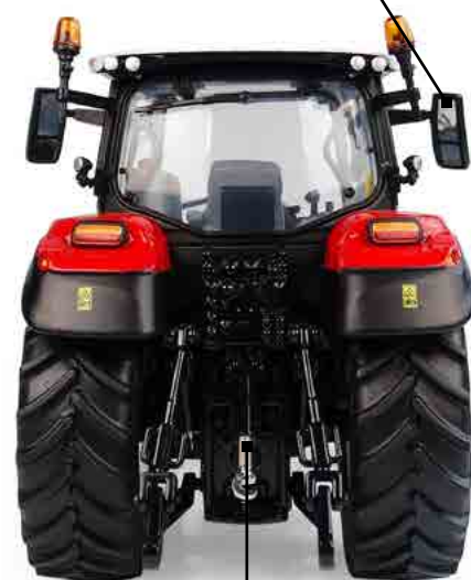
Adjustable third point linkage
