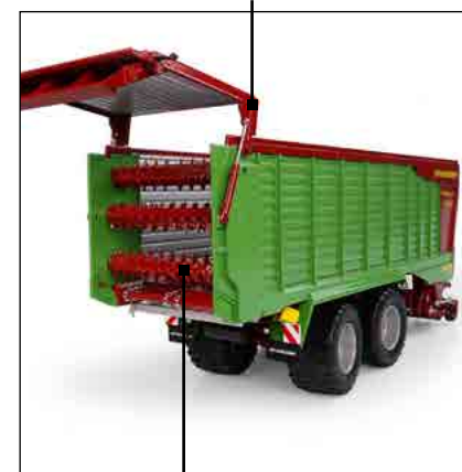
Assembly with 3 working drums with ripping tins
