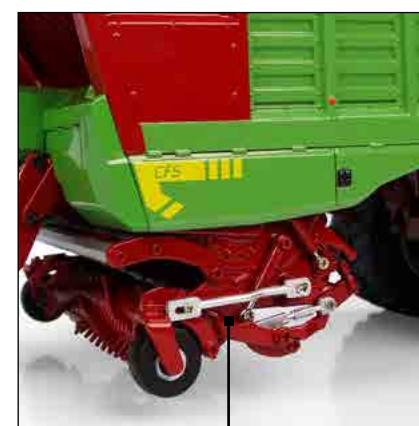
Adjustable pick-up height with turning wheels
