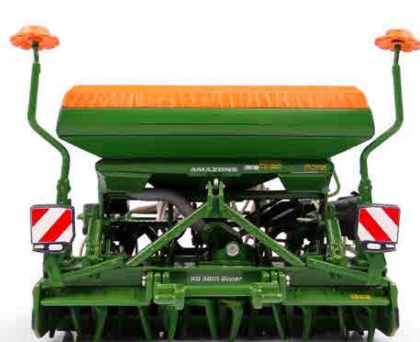
The Amazone KG3001 Super can be splitted from the Centaya harrow mounted seed drill
