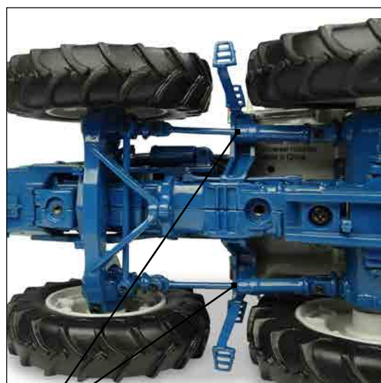
The 4 wheel-drive equal size wheel with the double transmission was main County 1147 feature
