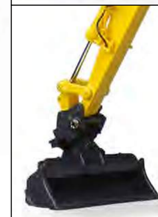
↗ KOMATSU PW148-10 with standard & ditch cleaning bucket UH8083
